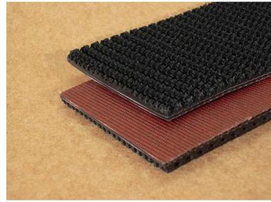
**Features:** This belt offers excellent gripping for standard incline conveyors. The polyester carcass offers high strength and low stretch. NOTE--The rough top impression must be recessed to use lacing. Use Recessed OAG for Lacing Recommendation.
